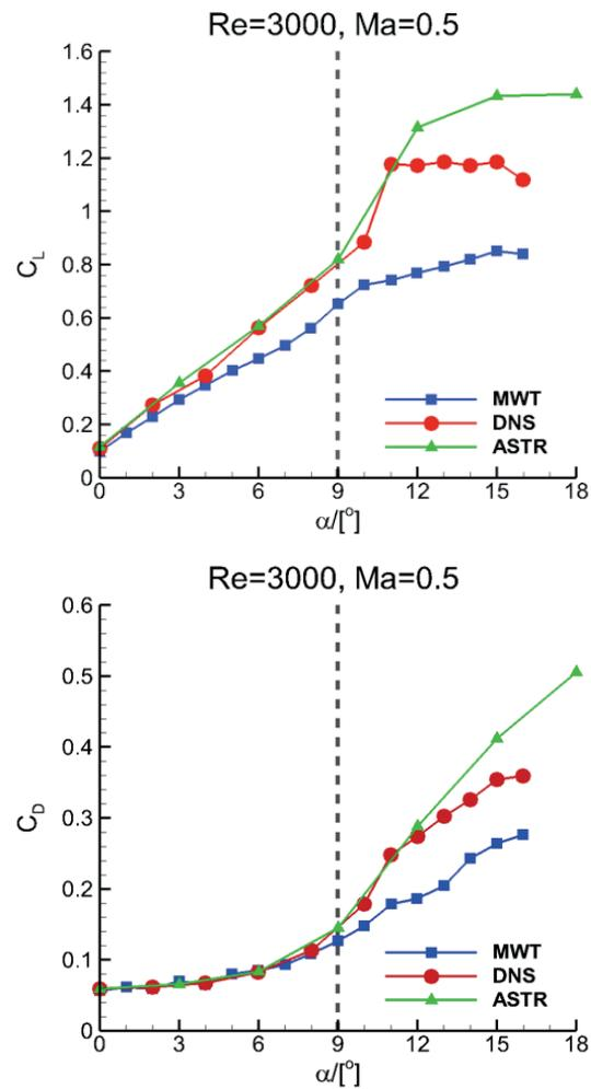
Figure 5. Comparison of time-mean force coefficients with the results from reference.
