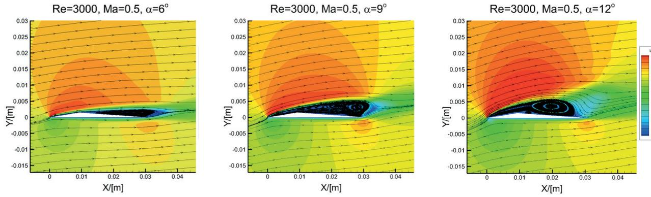
Figure 6. Time-mean flow fields with the contour of normalized velocity magnitude.
