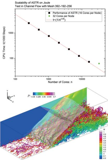
Figure 3. Scalability of ASTR and resolved structures in a supersonic turbulent flow by ASTR.
