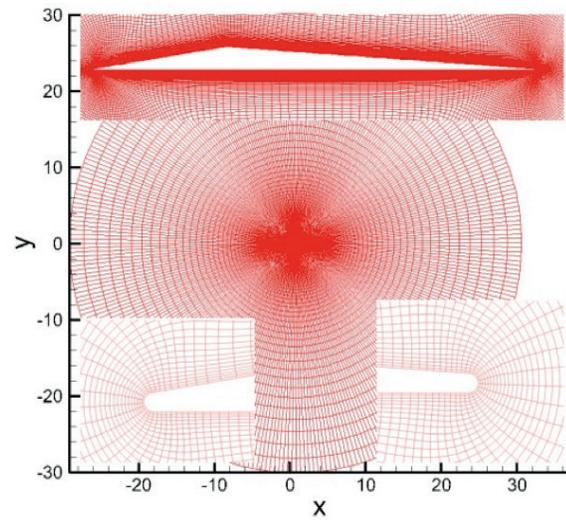
Figure 4. The O-type mesh used in the study.
