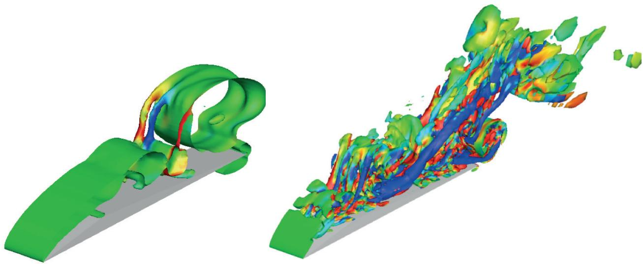
Figure 7. Instantaneous flow structures at  $Re=3,000$  (left) and  $Re=10,000$  (right).
